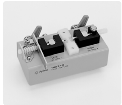
16034G Test fixture For SMD components.
